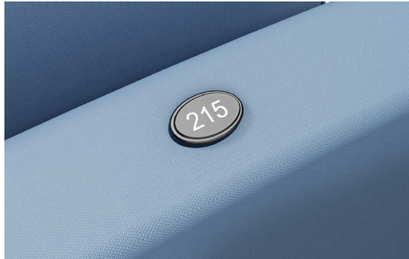
Seat Identification Polymer number plate placed with concealed fasteners. Font white Helvetica numbers Plate dimensions: 1" x 1 1/2" (26mm x 42mm) PA9712
